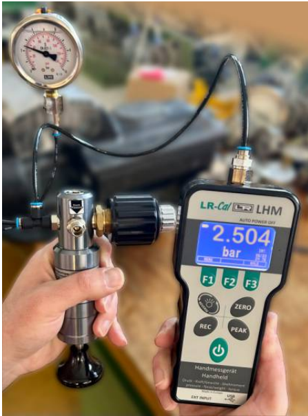
LR-Cal LHM with external pressure sensor LR-Cal LHM-TP16 and pneumatic pressure test pump LR-Cal LPP 10
