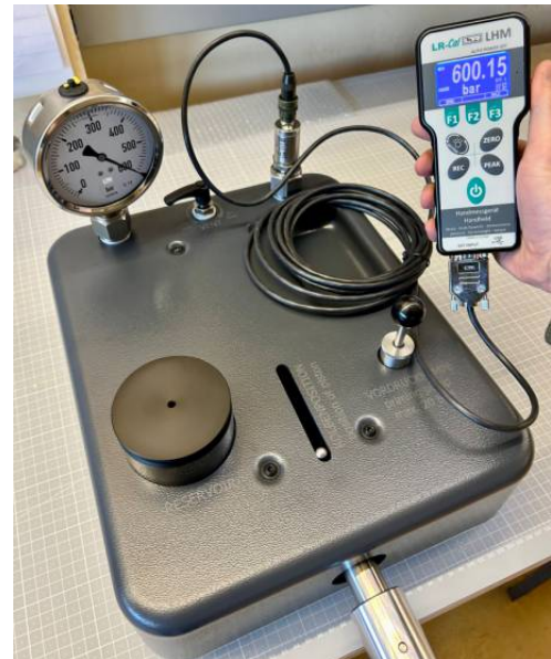
LR-Cal LHM with external pressure sensor LR-Cal LHM-TP16 and hydraulic pressure comparison test pump LR-Cal LSP 1000-H
