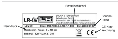
Fig. 1 manufacturing label (Nenndruck = nominal pressure; Bestellschlüssel = order code; Seriennummer = serial number; CE-Kennzeichnung = CE mark)
