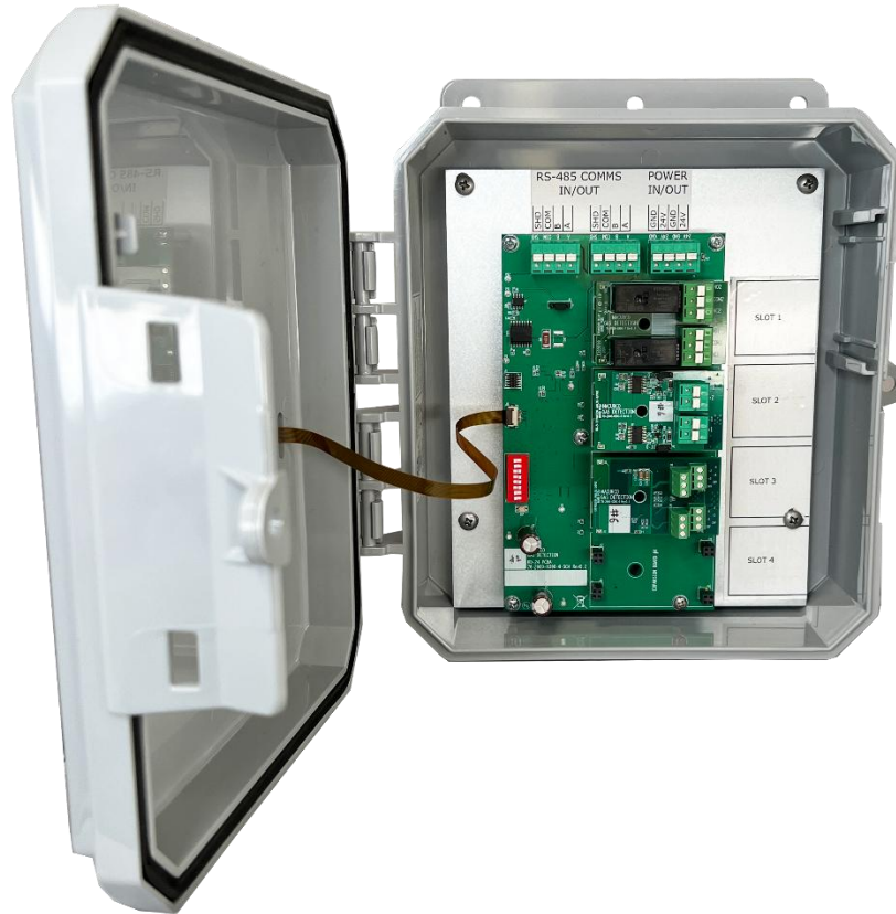
Figure 3-2 – Internal view with expansion boards
