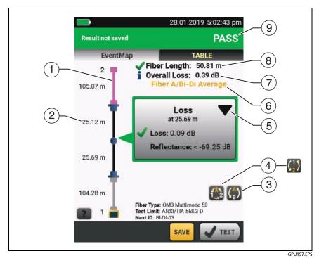
Figure 114. EventMap for Averaged, Bi-directional SmartLoop Results
