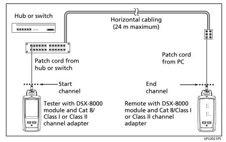
Figure 20. Channel Connections for Cat 8/Class I/II Links
