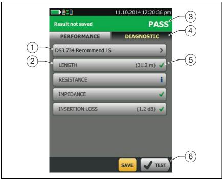
Figure 31. Autotest Results for Coaxial Cabling
