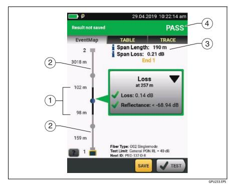
Figure 116. EventMap for a Span
