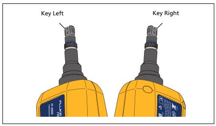
Figure 44. Key Position of the Tip
