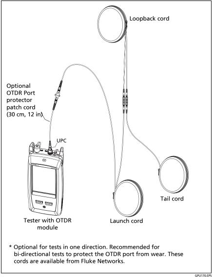
Figure 90. SmartLoop Launch Compensation Connections
