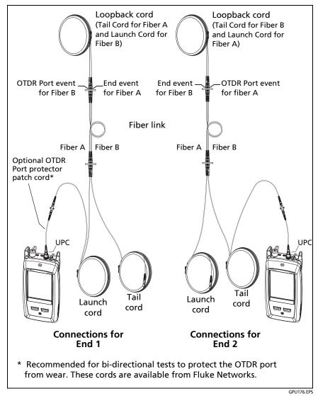
Figure 93. SmartLoop Test Connections for a Bi-Directional Test
