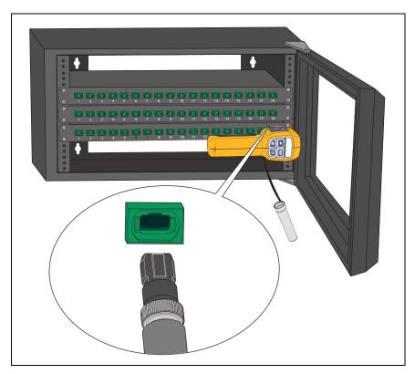
Figure 45. Key Left Position with Opposed Key Adapter
