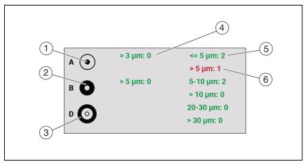
Figure 51. Defects Tab (Single Fiber shown)
