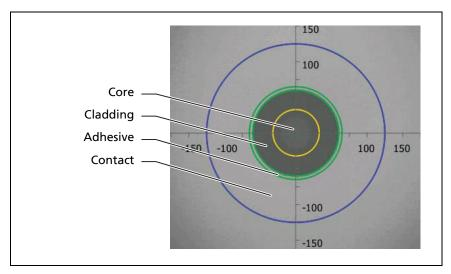
Figure 50. Zones on a Single Fiber Endface
