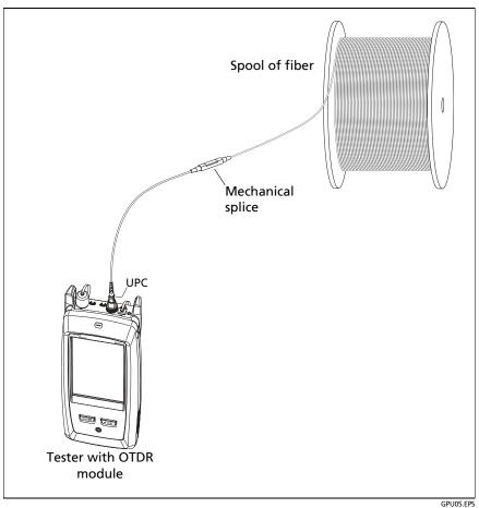
Figure 80. OTDR Connected to a Spool of Fiber
