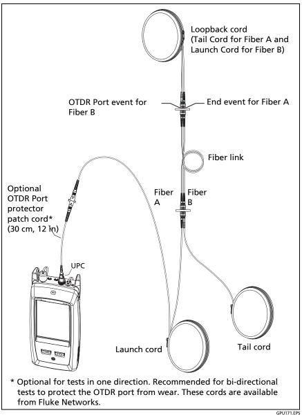
**Figure 91. SmartLoop Test Connections**
