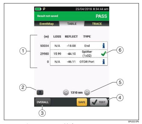
Figure 103. Event Table from an HDR OTDR Test
