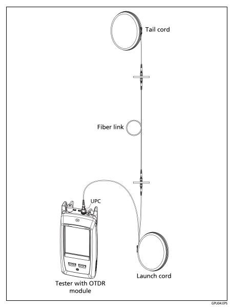
Figure 79. OTDR Connected with Launch and Tail Cords
