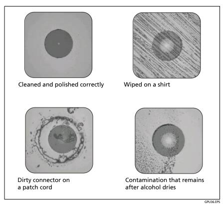
Figure 33. Examples of Clean and Dirty Fiber Endfaces
