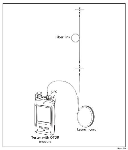
Figure 78. OTDR Connected with a Launch Cord
