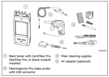
Figure 34. Equipment to Clean and Inspect Fiber Endfaces
