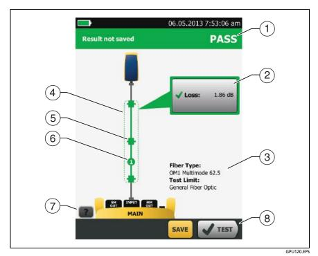
Figure 69. Result for Far End Source Mode
