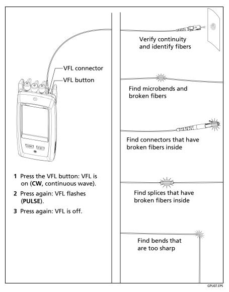
Figure 120. How to Use the Visual Fault Locator
