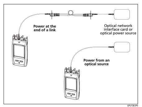
Figure 122. Connections to Monitor Power and Loss
