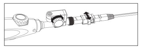
Figure 41. MPO/MTP® Inspection Tip
