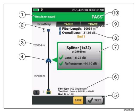
Figure 102. EventMap for an HDR OTDR Test Result
