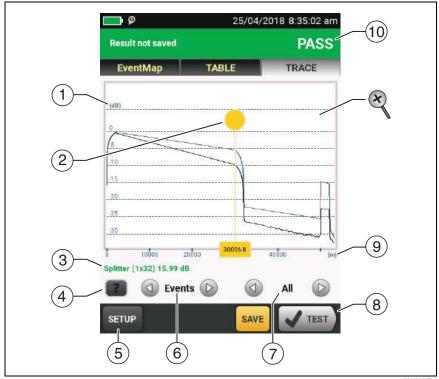
Figure 104. HDR OTDR Trace
