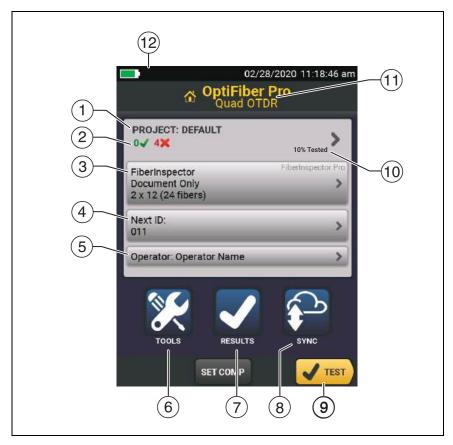
Figure 47. Home Screen for FiberInspector Pro Tests
