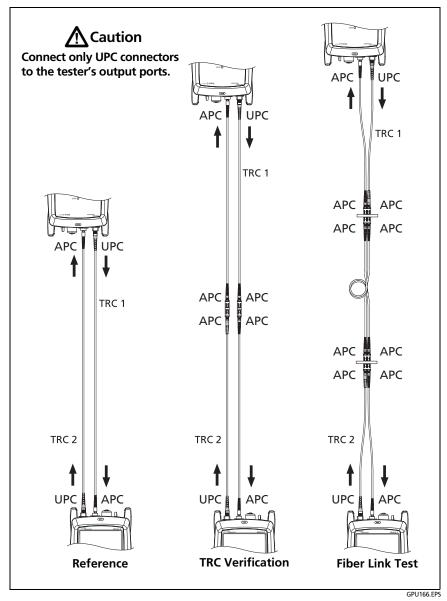
Figure 57. TRCs Necessary for Links with APC Connectors
