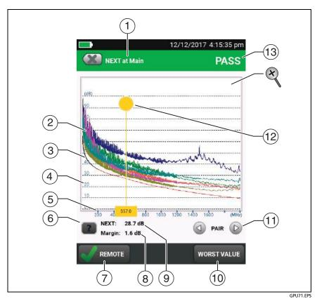
Figure 27. Plot Screen for a Frequency-Domain Test
