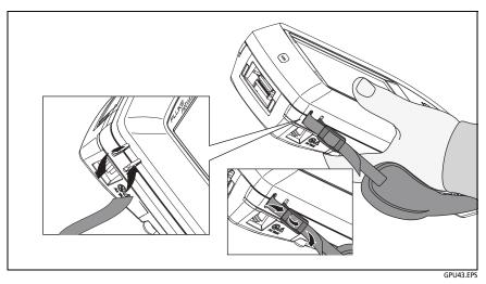
Figure 5. How to Install a Strap and Use the Hand Strap
