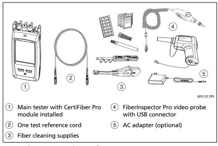
Figure 121. Equipment for Power Meter Measurements
