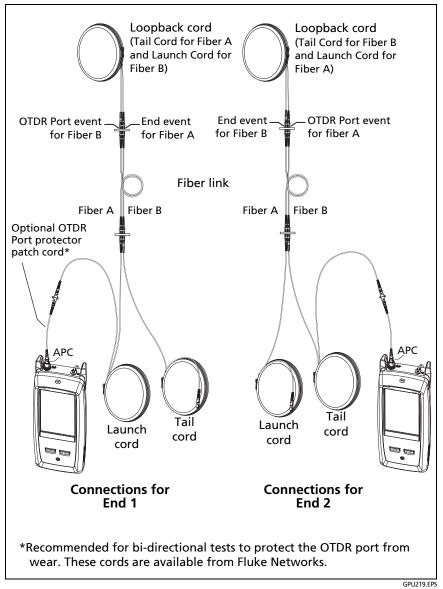
Figure 113. SmartLoop Test Connections for a Bi-Directional Test
