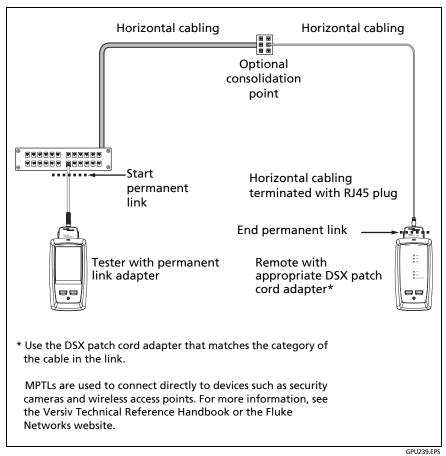
Figure 21. Connections for Modular Plug Terminated Links (MPTL)
