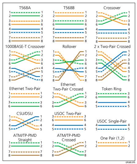
Figure 14. Outlet Configurations - RJ45
