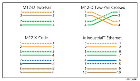
Figure 15. Outlet Configurations - Industrial Ethernet
