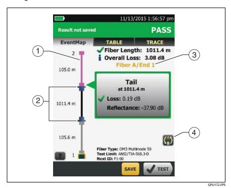
Figure 92. EventMap from a SmartLoop Test
