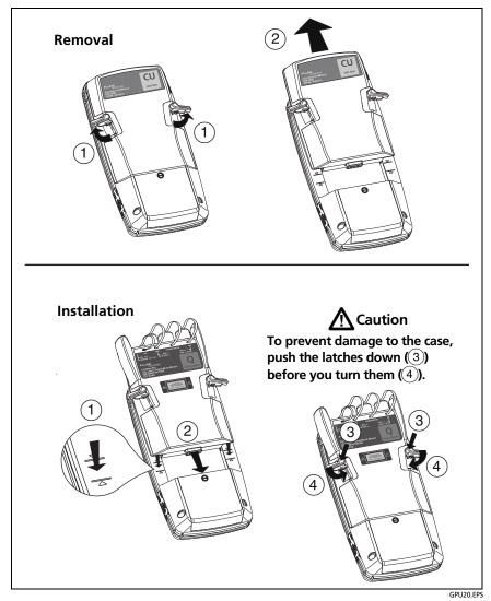
Figure 6. How to Remove and Install a Module
