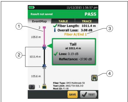
Figure 112. EventMap from a SmartLoop Test
