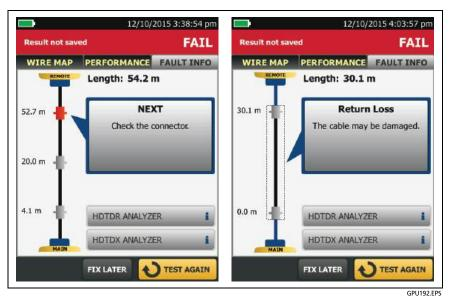
Figure 22. Examples of Fault Information Screens
