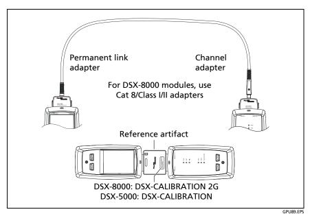
Figure 13. Reference Connections for Twisted Pair Cable
