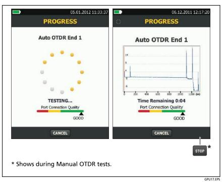
Figure 76. The OTDR Port Connection Quality Gauge and Progress Screen
