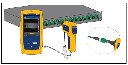
Figure 48. Inspect an Endface (FI-3000 shown)
