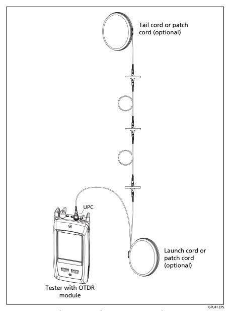
Figure 87. FaultMap Test Connections
