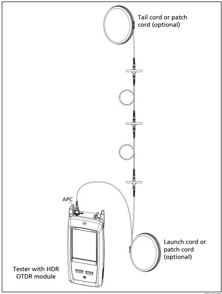
Figure 107. FaultMap Test Connections
