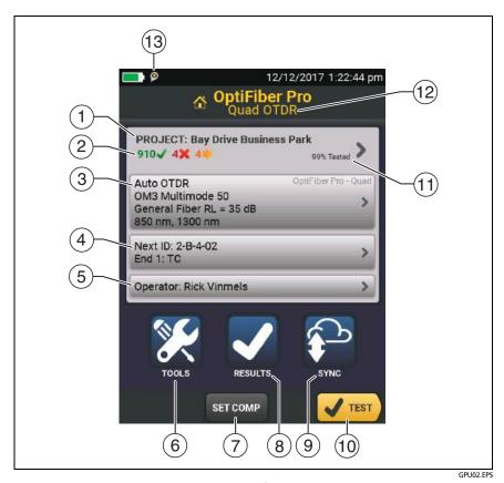
Figure 73. The Home Screen for OptiFiber Pro Modules
