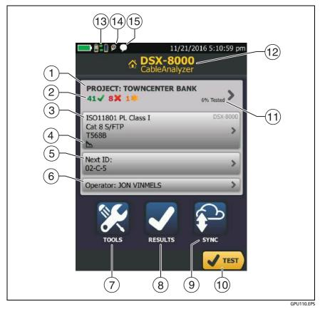
Figure 12. The Home Screen for the DSX CableAnalyzer
