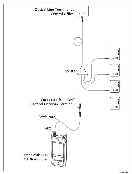
Figure 100. Typical Connections to an Out-of-Service PON Link
