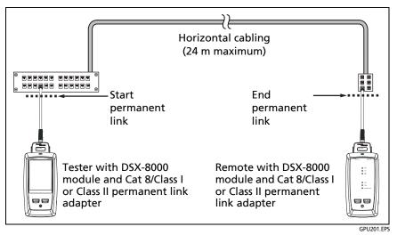
Figure 19. Permanent Link Connections for Cat 8/Class I/II Links
