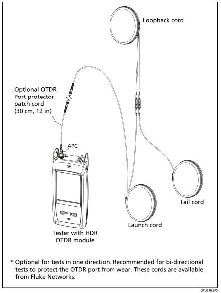
**Figure 110. SmartLoop Launch Compensation Connections**
