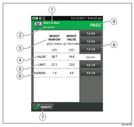
Figure 26. Tabular Results Screen for a Frequency-Domain Test
