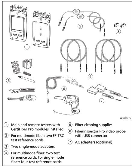
Figure 60. Equipment for Autotests in Smart Remote Mode
