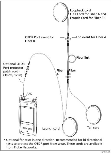
**Figure 111. SmartLoop Test Connections**
