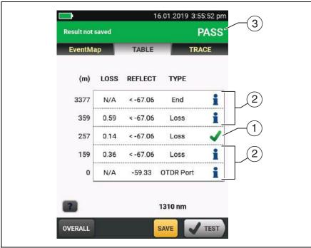
Figure 117. Event Table for a Span
