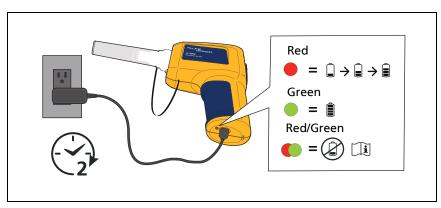
Figure 39. Charge the Battery
