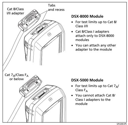
Figure 11. DSX-8000 and DSX-5000 Module and Adapter Differences
