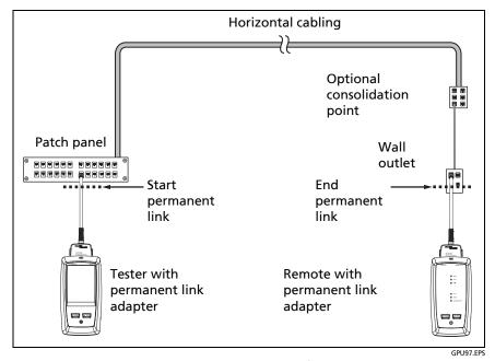
Figure 17. Permanent Link Connections for Links Up to Class  ${\bf F}_{\bf A}$
