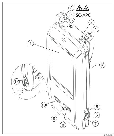
Figure 95. Connectors, Keys, and LEDs (Versiv 2 with OFP-200-S1625 OTDR module shown)
