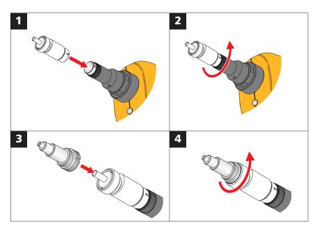
Figure 42. Single Fiber Tip Attachment
