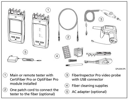
Figure 119. Equipment for Visual Fault Locator Tests
