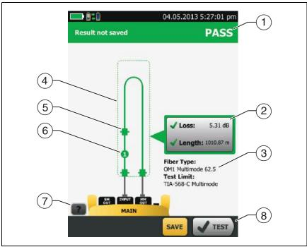
Figure 65. Result for Loopback Mode
