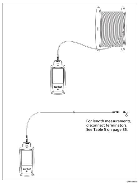
Figure 32. Connections for Coaxial Tests Without a Remote
