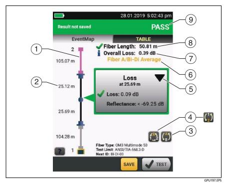
Figure 94. EventMap for Averaged, Bi-directional SmartLoop Results
