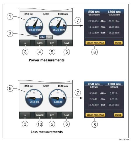
Figure 123. Power Meter Measurements and Controls
