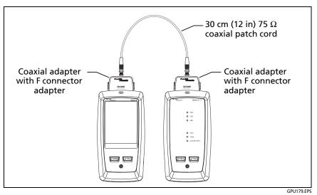
Figure 28. Reference Connections for Tests on Coaxial Cabling
