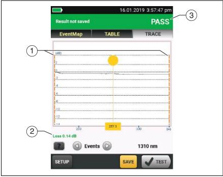
Figure 118. OTDR Trace for a Span
