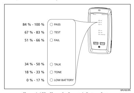
Figure 1. LEDs Show the Remote's Battery Status
