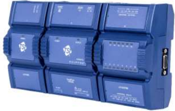
Figure 1: Laboratory Room Controller
