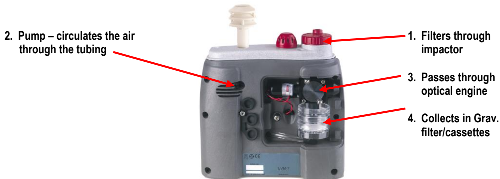
Figure 4-3: How the impactor functions
