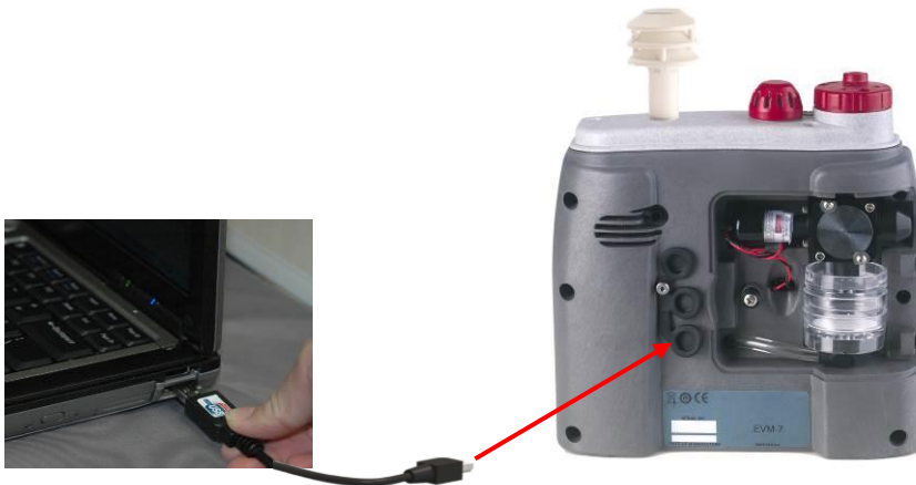
Figure 2-7: Communicating with DMS via USB cable
