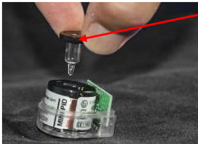
Figure 7-6: Fitting/Inserting the lamp and pellet
