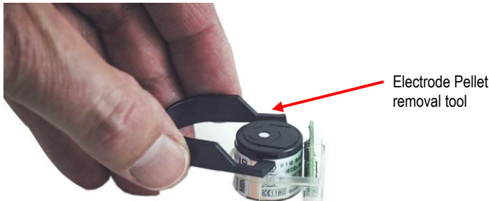
Figure 7-3: Removing the lamp with removal tool
