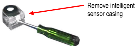
Figure 7-2: Removing intelligent-sensor casing with PID
