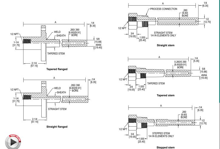
Series W Thermowells select bore as 0.260 for 1/4" diameter elements and 0.390 for 3/8" diameter elements. Specify heavy duty mounting for tapered sheaths.
