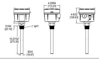
The Model VRLS Vibrating Rod Level Switch is economical choice in level detection of powders and bulk solids. The VRLS incorporates a piezoelectric crystal that vibrates the rod at its natural frequency, when contact material is present it dampens the vibrations and the switch changes state.
