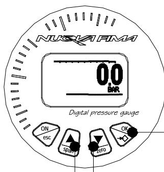
Use UP and DOWN keys to select the desired menu page, as shown in the figure, and press OK
