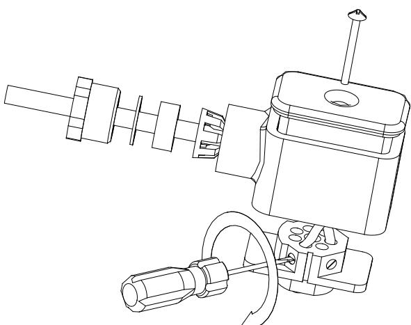
2 – Connect cable (see figure) remount the connector and fix it on the instrument
