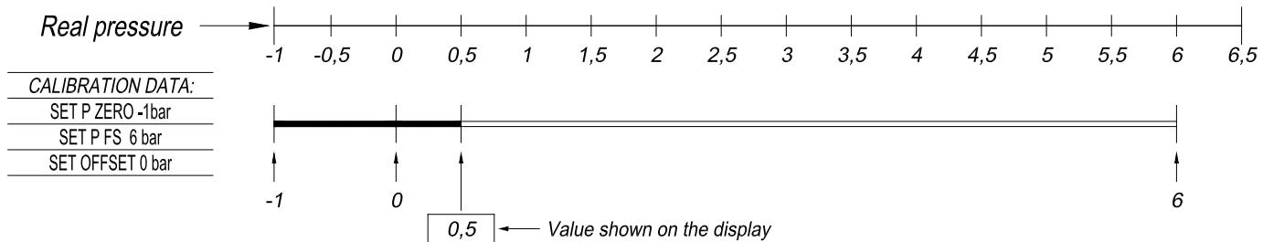
For error correction key in -0,5 bar in the window dialogue SET P OFFSET
