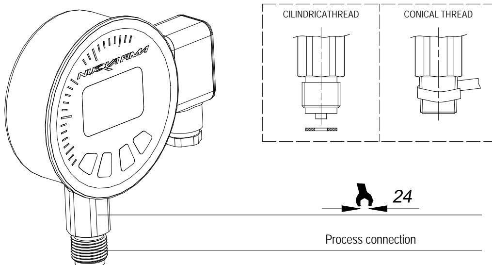
If the instrument is equipped with a fluid separator, the grip by which to tighten the attachment, must be carried out on the latter and not on the instrument itself, as this may affect calibration.
