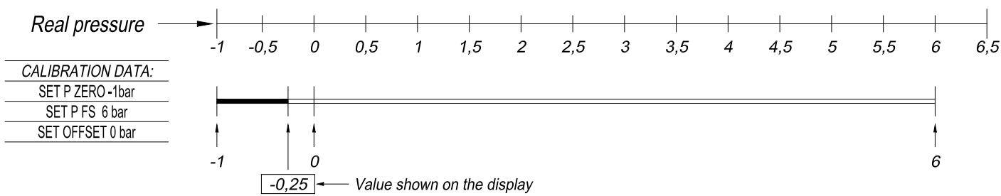
For error correction key in -0,25 bar in the window dialogue SET P OFFSET
