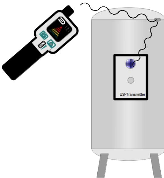
For example Leak test at a tank:
