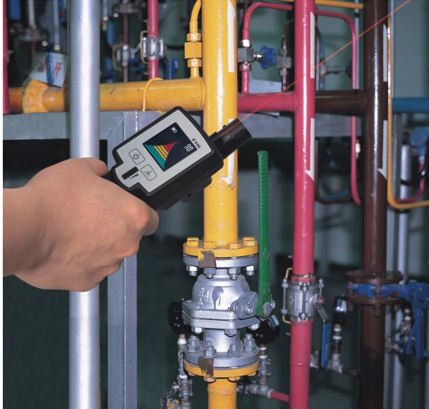
3. To activate the laser, please press the button which is shown on the left side.
