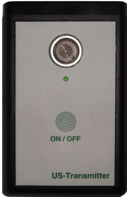
The Ultrasonic tone generator is an optional extra accessory for the S530. It generate an ultrasonic tone which can be detected by the S530. Thats why a leak detection in a system without overpressure is possible.
