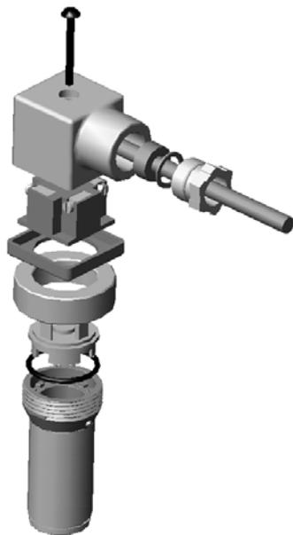
Figure 1 – Exploded view of the connector
